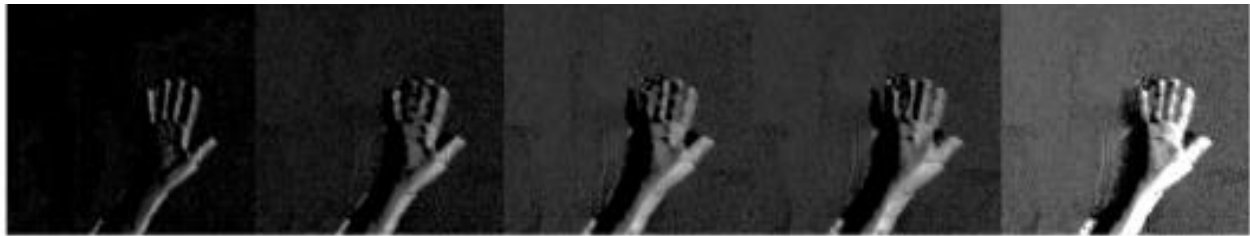
Figure 2: Example of hand motion identification where the moving item, such as the hand, is recovered from a stationary backdrop using frame difference calculation to get hand characteristics
