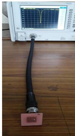
Figure 11: Measurements carried out in VNA
